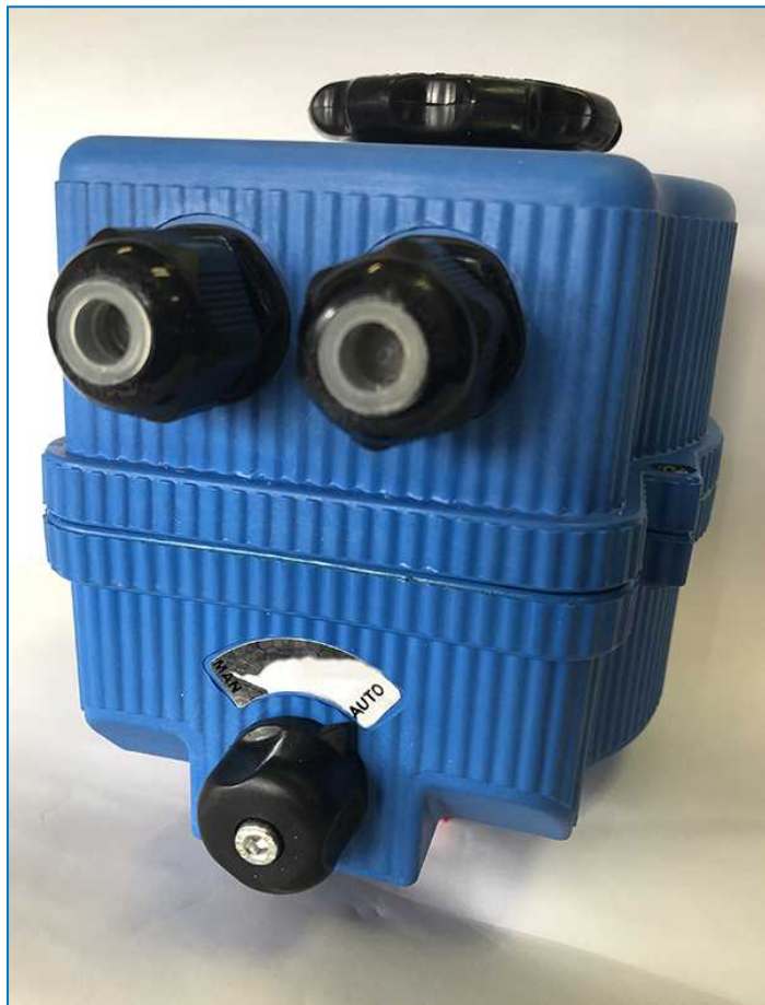
Purge valve actuator position "AUTO"
