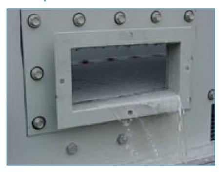
A factory-installed clean out port
