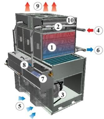
When a module works **dry**, the spray pump is turned off. Heat is now transferred from the process fluid to the ambient air using sensible heat transfer.
